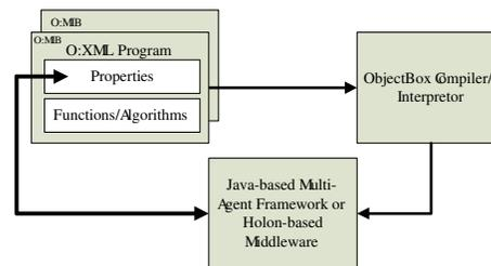
Figure 5. Integration of Multi-Agent Framework with O:XML-Implemented O:MIB
