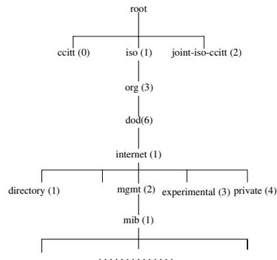
Figure 1. The Functional Domain of O:MIB in MIB Tree Structure
