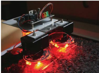
Fig. 2. Experimental test setup with two optical mouse sensors on gantry mounted above road surface
