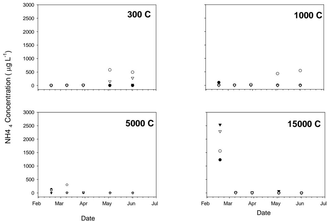
**Figure 2. Ammonium response to different salt additions. Each point represents an individual mesocosm (C = constant salinity).**
