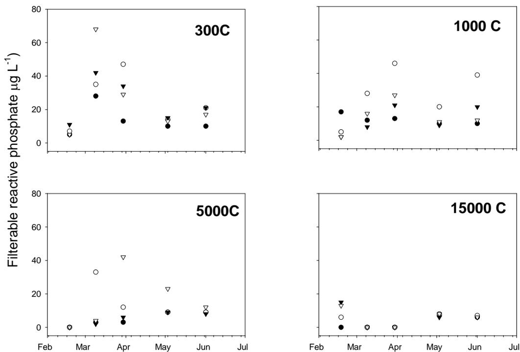
**Figure 3. Phosphate (as filterable reactive P) response to different salt additions. Each point represents an individual mesocosm (C = constant salinity).**
