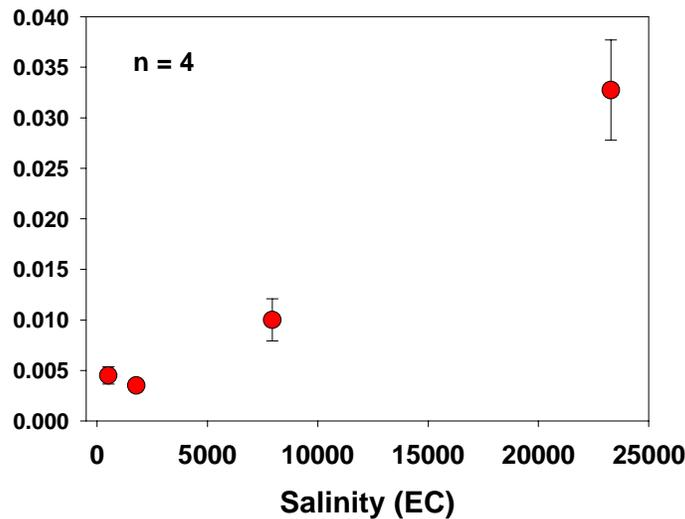
**Figure 6. Formation of acid volatile sulfur (Iron sulfide) in response to increasing salinity.**
