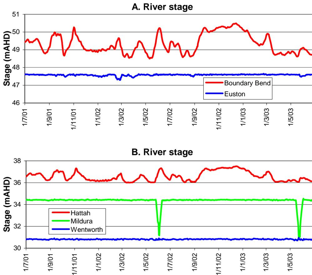
**Figure 3. River stage at (A) Boundary Bend and Euston, and (B) Hattah, Mildura and Wentworth from July 2001 – June 2003. For weirs, gauges were located immediately upstream of the structures.**
