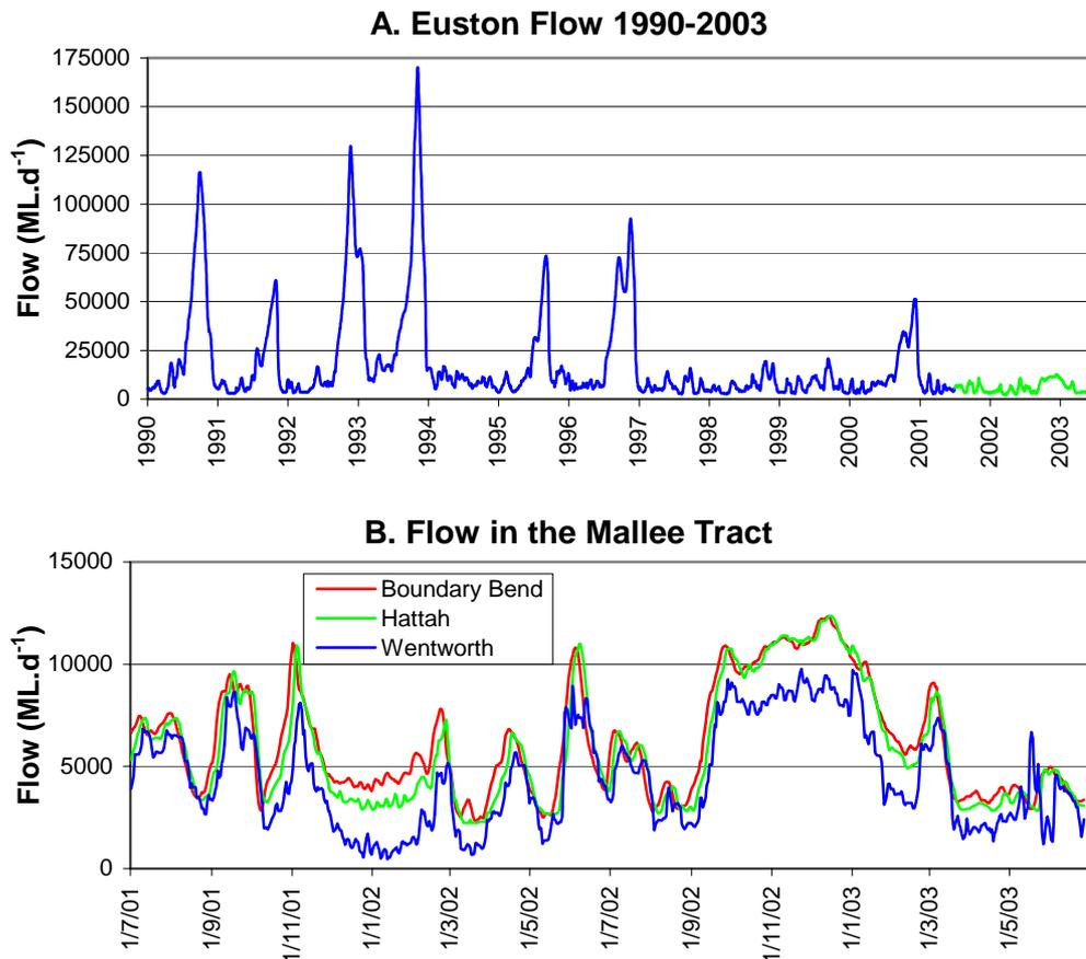
Figure 2. Daily flow at (A) Euston from 1990-2003 (two-year study period highlighted in light green), and (B) at Boundary Bend, Hattah (Colignan gauge) and Wentworth from July 2001 - June 2003.
