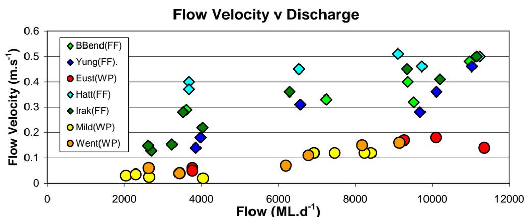
**Figure 4. Flow velocity v discharge relationships at seven riverine sites within the study reach.** Note the different relationships between the weir pool (circles) and free-flowing (diamonds) sites.
