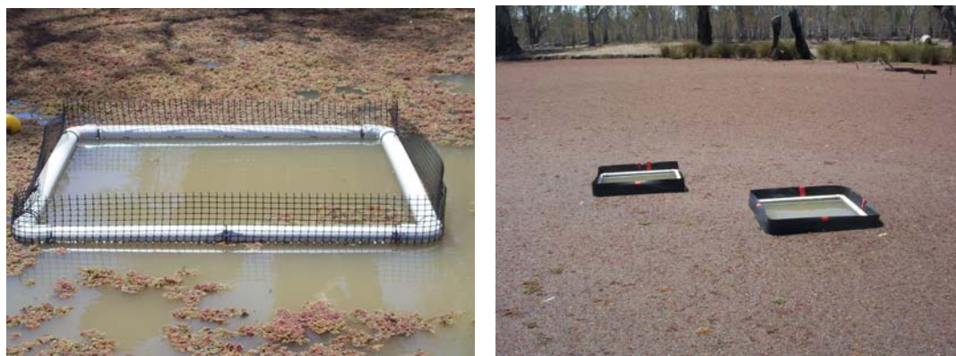
Figure 1. Growth enclosures designed to allow in situ measurement of Azolla growth rates.
