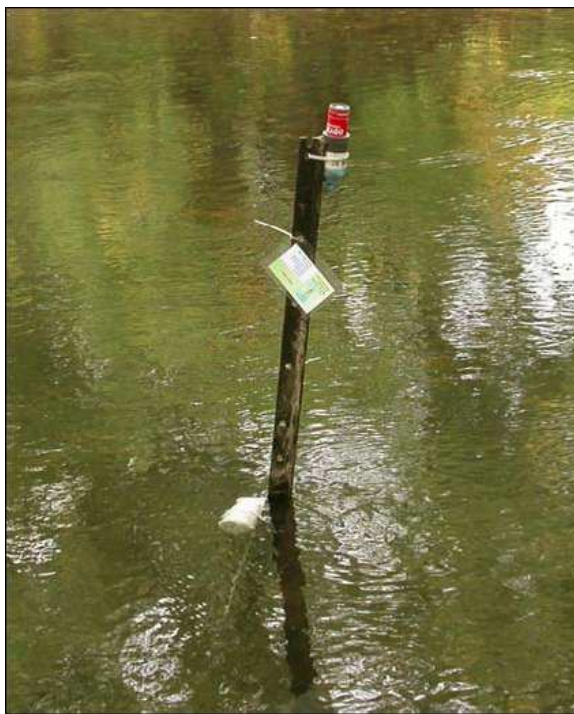
Figure 2. Water temperature logger (A) and light logger (B) deployed in the Ovens River (Gawne et al. 2005)
