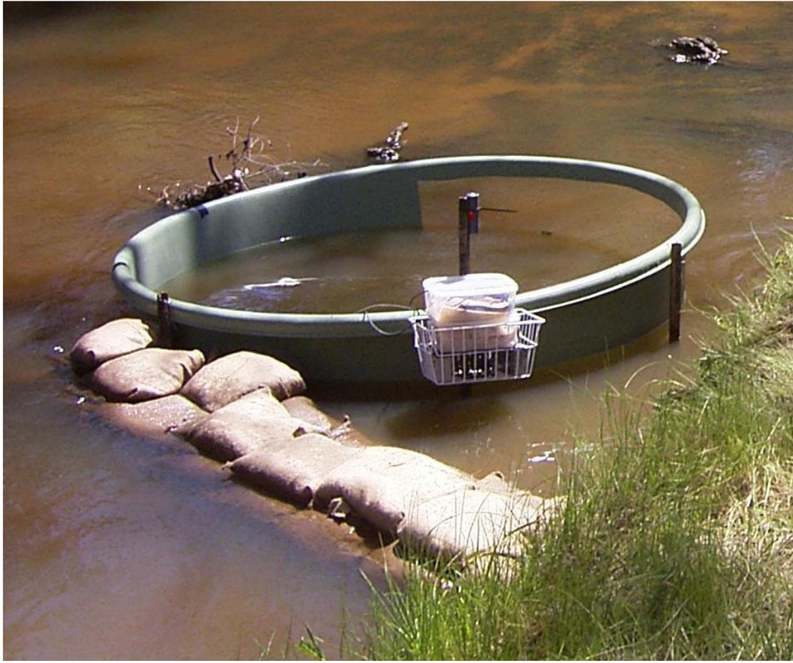
**Figure 2.** Tank installed to create a slackwater.
