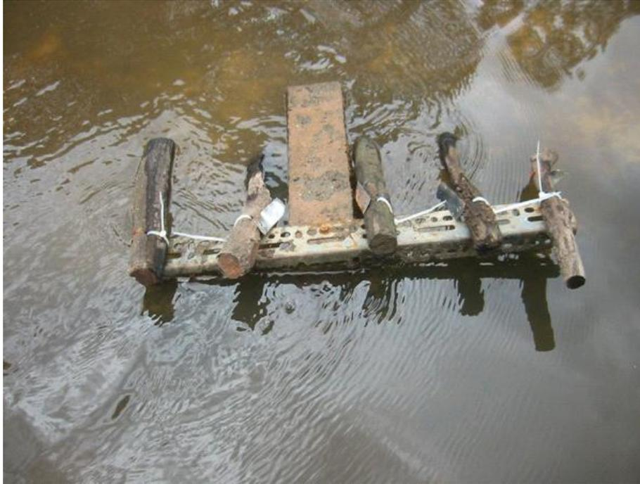
**Figure 3.** Platform sampler for snag segments.
