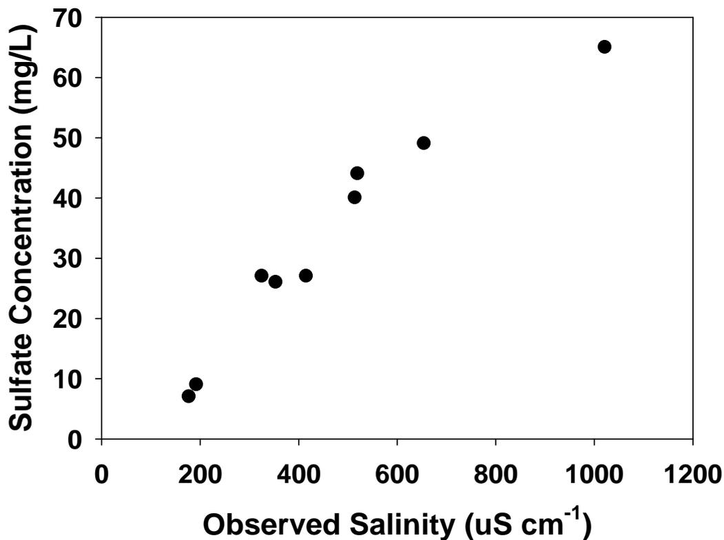
Figure 3 - Relationship between sulfate in the water column and measured electrical conductivity
