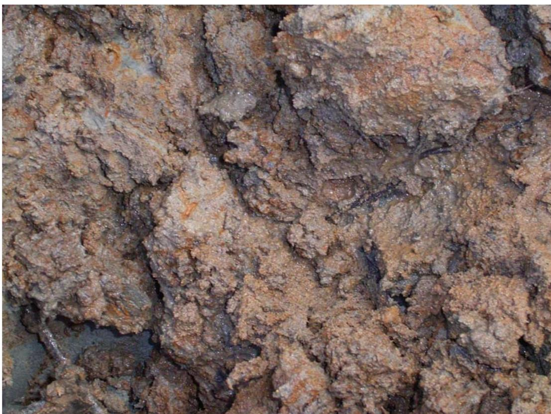
Figure 4 - iron mottling evident at Site k
