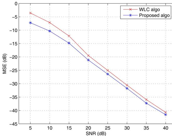
Fig. 2. Comparison of the proposed algorithm with the WLC algorithm in the presence of virtual carriers. One block of data used in both methods.
