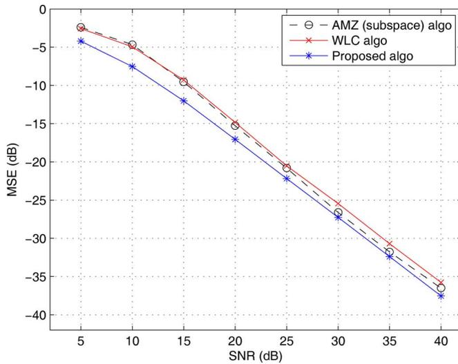
Fig. 1. Performance comparison of the proposed algorithm with WLC and (subspace-based) AMZ algorithms. One received data block used for the proposed and WLC algorithms. Forty data blocks used for the AMZ algorithm.
