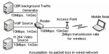
Figure 2a: Simulation setup (one mobile receiver node)
