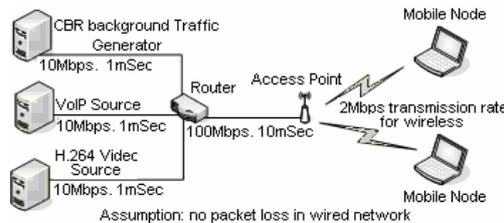
Figure 2b: Simulation setup (2 mobile receiver nodes)
