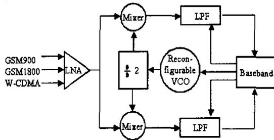
Figure 5. Multistandard receiver architecture with VCO
