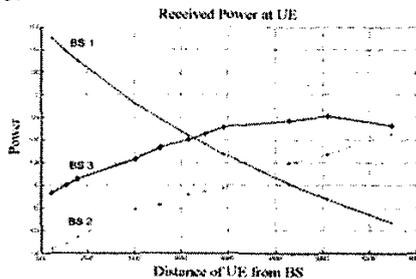
Figure 3. Received power at UE from base stations
