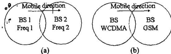
Figure 1(a) Inter-frequency handover, (b) Inter-system handover
