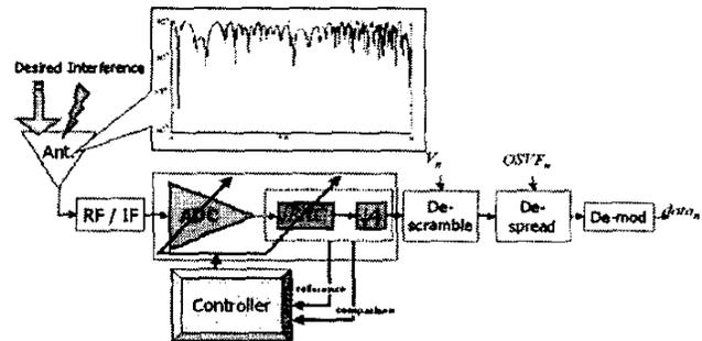
Figure 2. UTRA-TDD Mobile Station Receiver Block Diagram [3]
