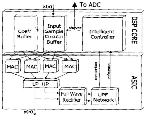
Figure 5. Reconfigurable Digital Filter Architecture
