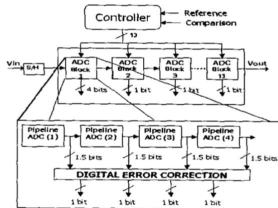
Figure 6. Reconfigurable Pipeline ADC System
