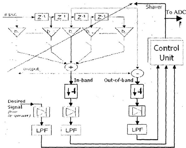
Figure 3. Reconfigurable Digital Filter System
