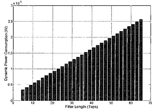
**Figure 7.** Dynamic Power Consumption of ASIC components in filter (clock = 15.36MHz)
