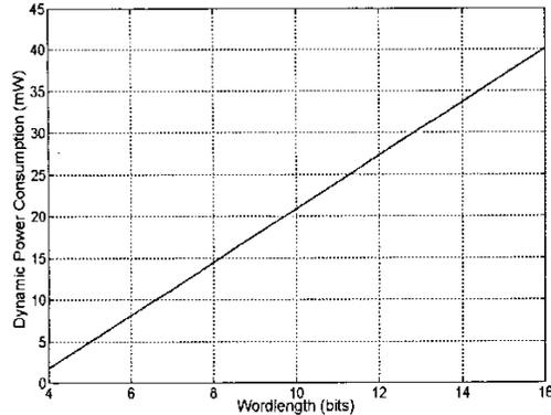
**Figure 7.** Dynamic Power Consumption of ASIC components in ADC (clock = 15.36MHz)
