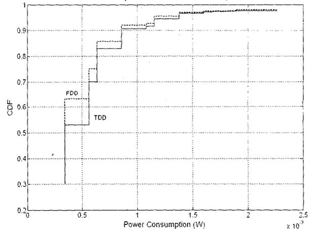
Figure 8. CDF of Dynamic Power Consumption of channel filter for UTRA-TDD/FDD (ex Control Unit)
