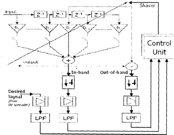
Figure 6. Channel filter with a scalable filter length
