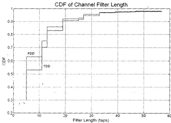
Figure 5. CDF of filter lengths for UTRA-TDD/FDD
