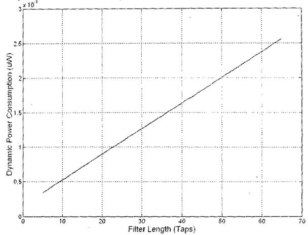
Figure 7. Dynamic Power Consumption of channel filter (ex Control Unit)
