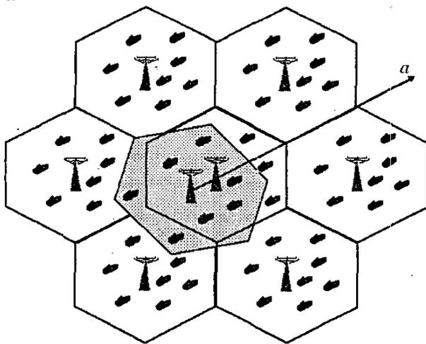
Fig. 4. Cell topology where multiple cells are causing ACI at a target cell on top of the interference cell cluster.
