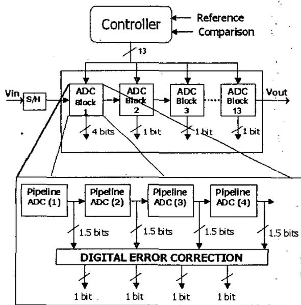
Fig. 8. Reconfigurable Pipeline ADC System
