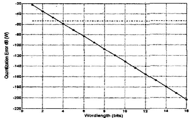
Fig. 7. Quantisation Error vs. Word Length
