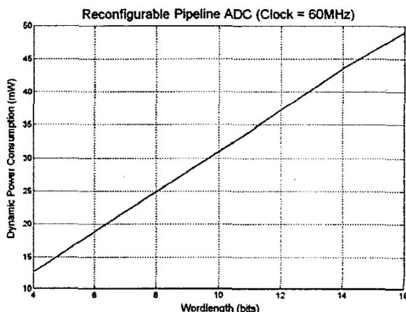
Fig. 9. Power Consumption for various word lengths (excluding DSP)
